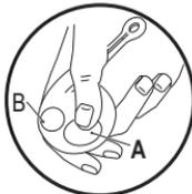
To disarm the system press the door unlocking pushbutton of the vehicle original remote control or, if the system is provided with it, the "B" pushbutton of the Cobra remote control.
